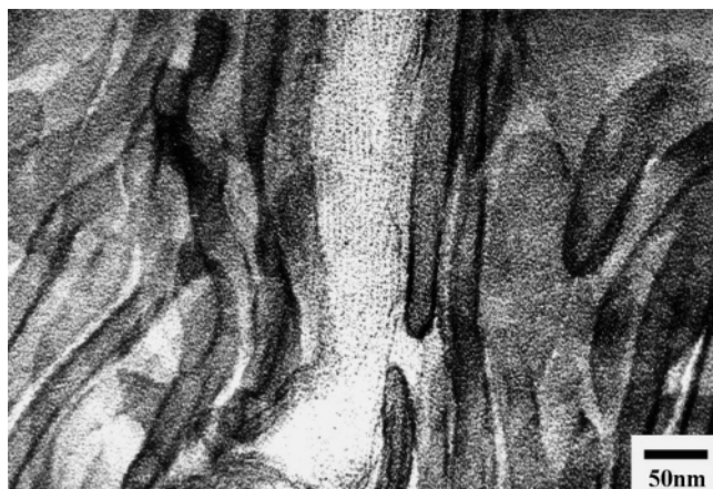
Figure 6. TEM micrograph of PCL3/PS-PEP blends. In the middle region of the TEM micrograph, alternate white and black thin stripes of PCL components are in between of PS-PEP component appeared as multilayer-like crystals.
